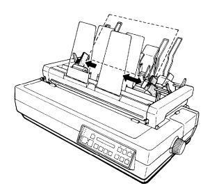
3. Take a stack of paper and fan it. Next, tap the paper on a flat surface to even up the stack.
